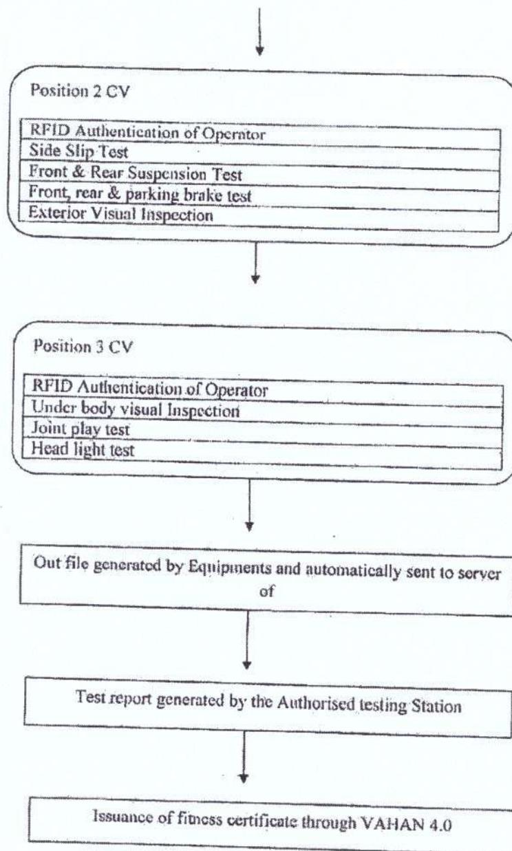
Note:- All result on the computer are hidden. No operator/Inspector is able to see the result of the vehicle weather it is pass/fail. No human intervention.
